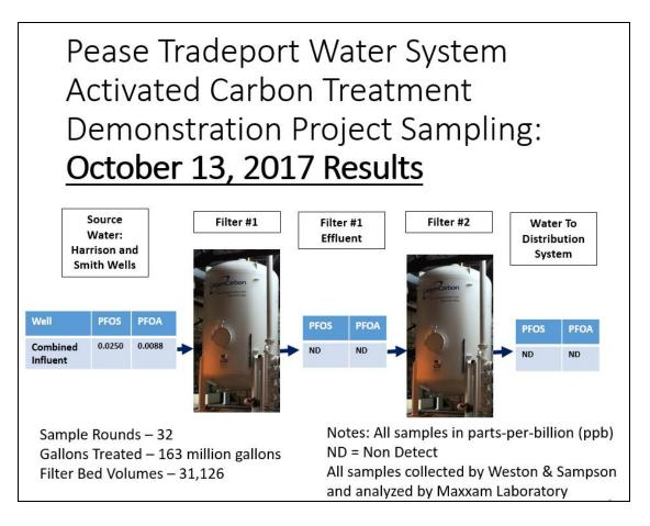
The activated carbon demonstration filters for the Harrison and Smith wells have been on line for over a year. As of October 13, 2017, 163 million gallons of water from these two wells has been treated through the activated carbon F400 Calgon Filtrasorb Filter media. This equates to 31,126 filter bed volumes of water.
